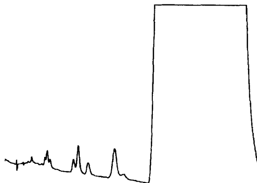
Fig. 2. HPLC chromatogram at 314 nm after irradiation at 25 kGy. Mobile phase: \text{KH}_2\text{PO}_4 0.05 M/ \text{CH}_3\text{CN} (98:2 v/v). Column Waters \mu -Bondapak (300 \times 3.9 mm).
